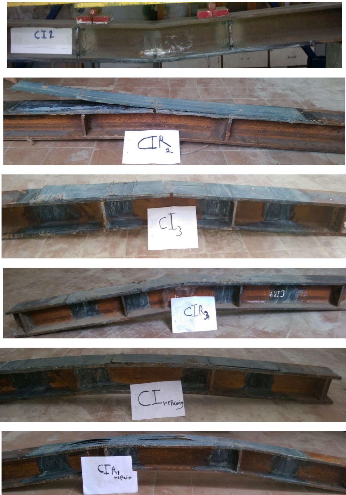
Fig.4. the shape of failure for the carbon under static and fatigue loads in the repairing cases.
